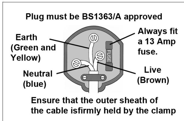
**We strongly recommend that this machine is connected to the mains supply via a Residual Current Device (RCD).**
